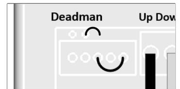
**DeadMan Function:** You use only the UP and DOWN buttons. You have to hold the button to make the lift move. When you release the button the equipment will stop immediately. If a key gets jammed you can stop the equipment with the stop button.
