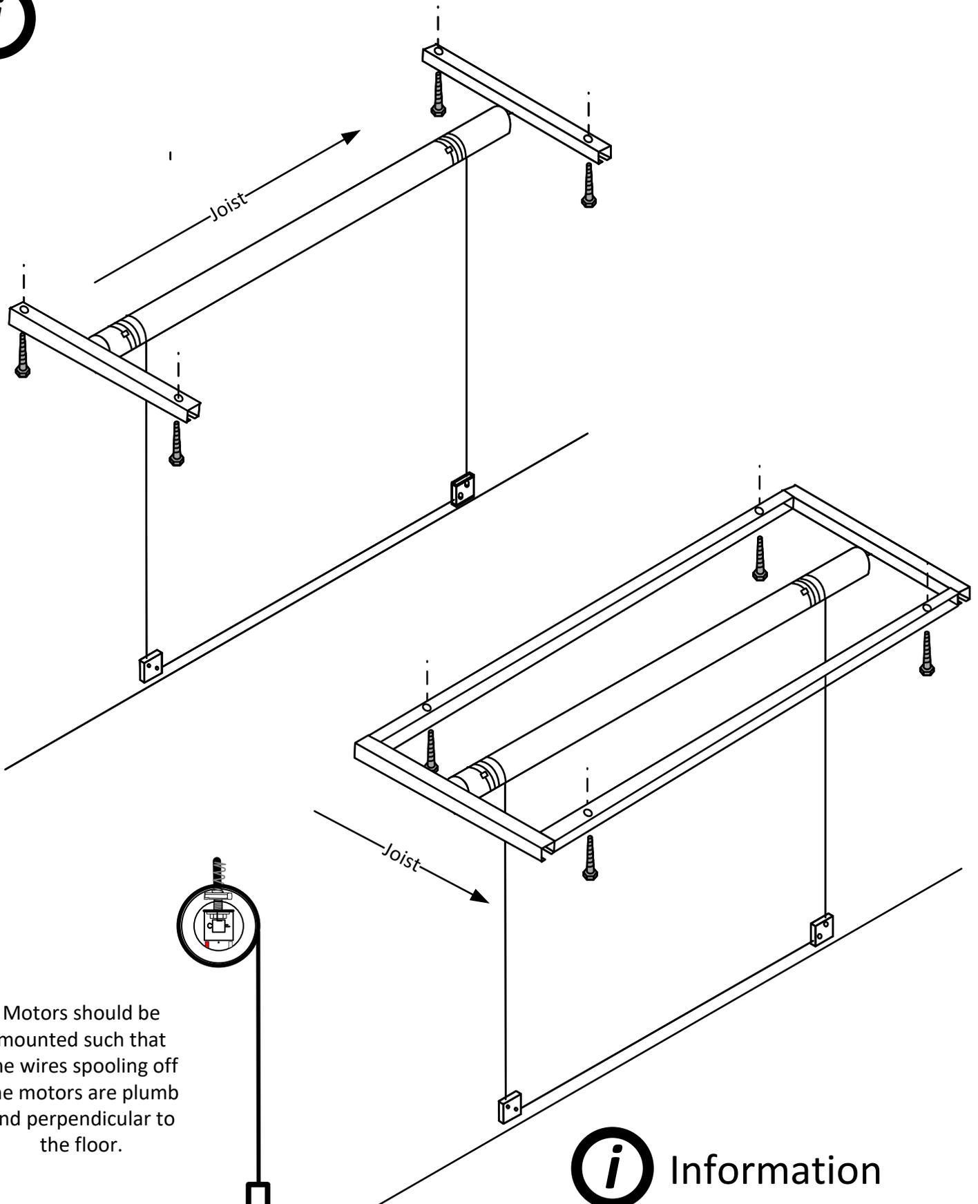
Motors should be mounted such that the wires spooling off the motors are plumb and perpendicular to the floor.
