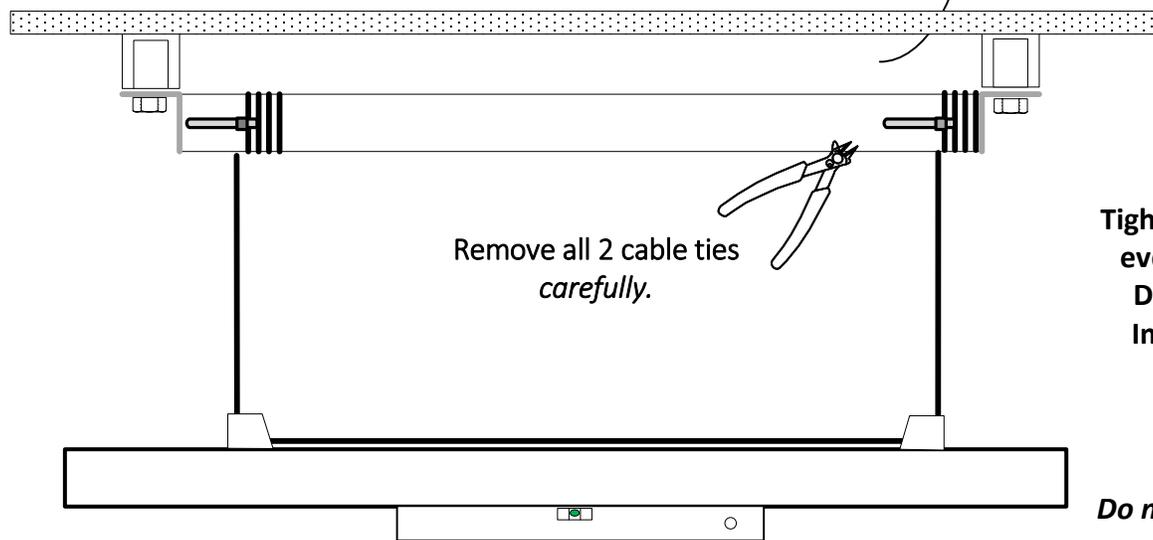
**Tighten the screws evenly by hand. Do not use an Impact driver.**
